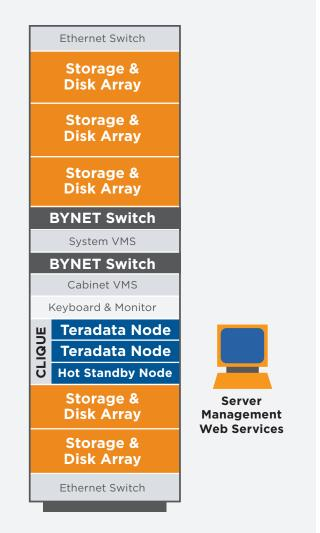
Figure 1. Teradata Active EDW 6700 Platform Cabinet Components.
